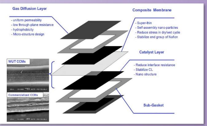
7-layer MEA structure. Photos on the left highlight the enhanced catalyst binding to the membrane, as compared to those produced by conventional technology
