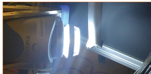
Alcon傳感器獲取點蝕的三維模型 Alcon sensor captures the 3D model of pitting
