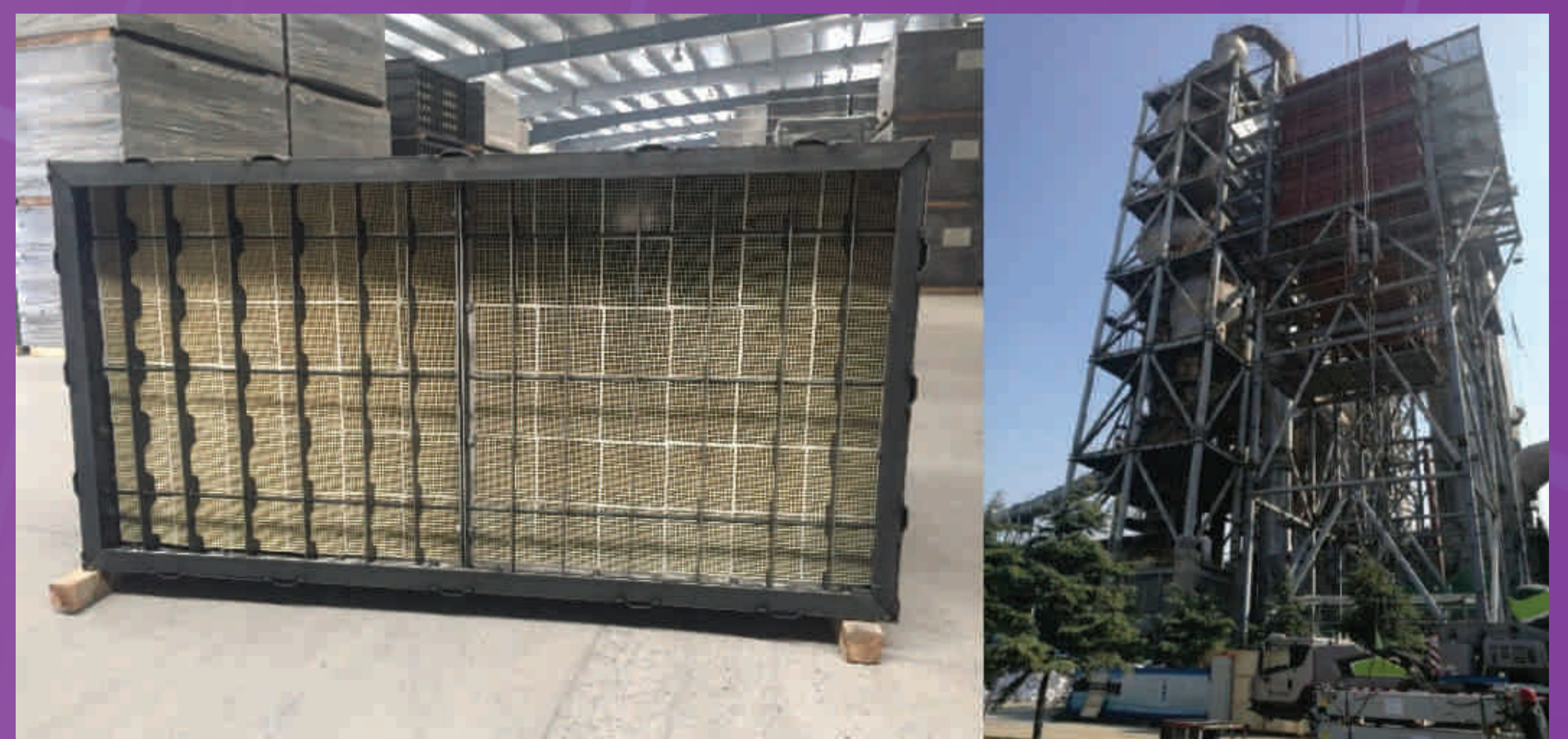
The standard catalyst model and the application of catalyst in industry. The catalyst has been successfully utilized in the industrial fields of steel, cement, glass, ceramics and garbage incineration power plant
