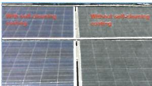
The comparison between the PV modules with and without self-cleaning coatings
