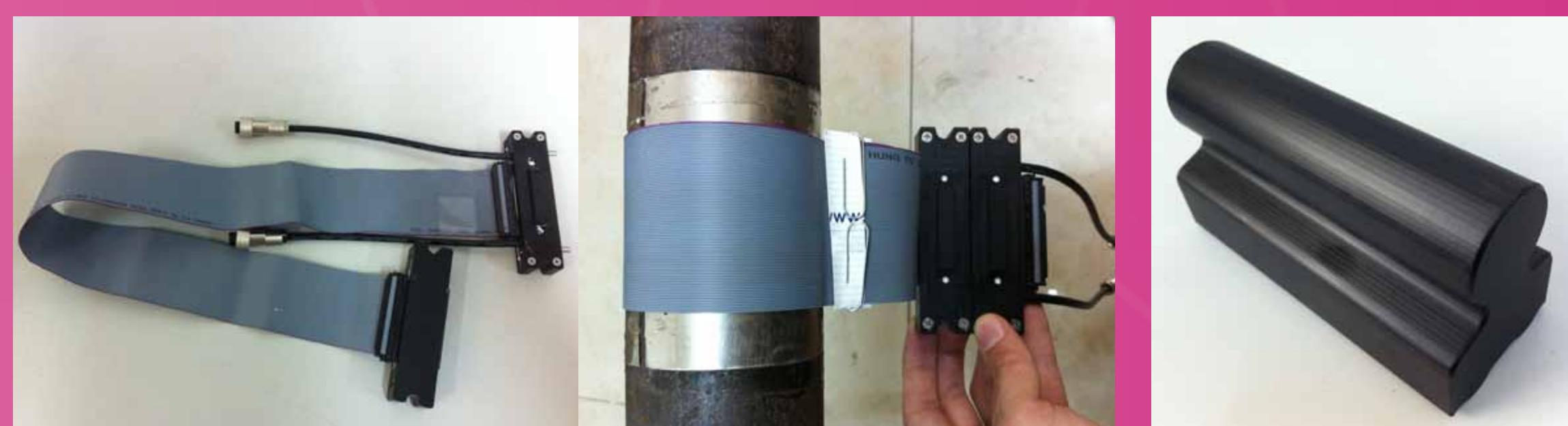
The transmitting-receiving probe installed on pipeline
