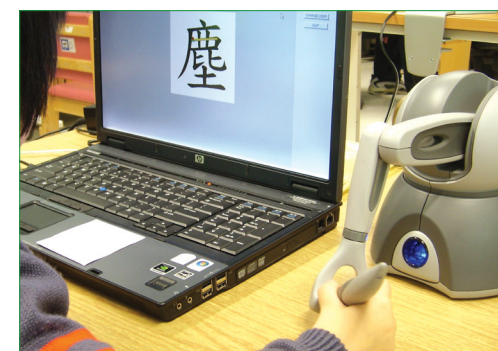
用來進行寫字訓練的觸感仿真平台 The haptic platform implemented for handwriting training
