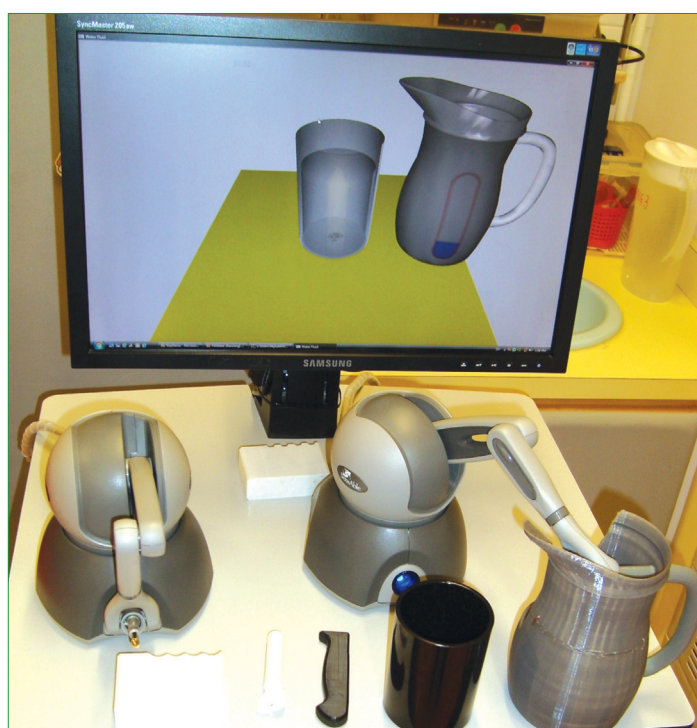
適用於自理培訓的觸感仿真平台的原型 The prototype of the haptic platform implemented for self-care training
