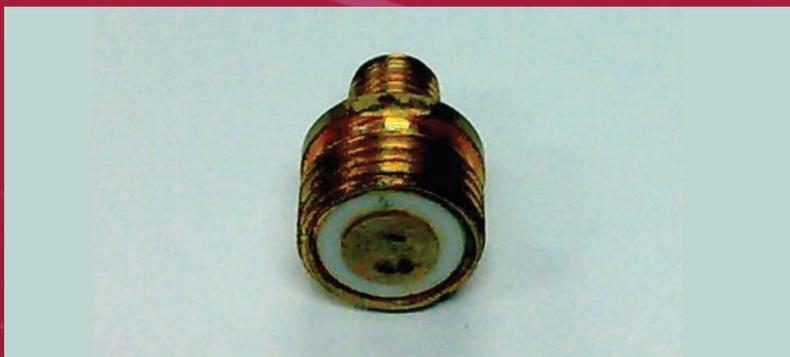
*Wear particles online electrostatics sensor*
