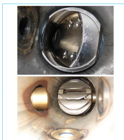
安裝在水管內的噴嘴和葉輪， 入水口（上圖）和出水口（下圖） The nozzle and impeller installed inside the pipe, viewed from the water entry (top) and water exit (bottom) side respectively
