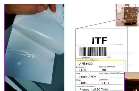
應用實例：RFID空運提單標籤 FRED application example: RFID-enabled air waybill label
