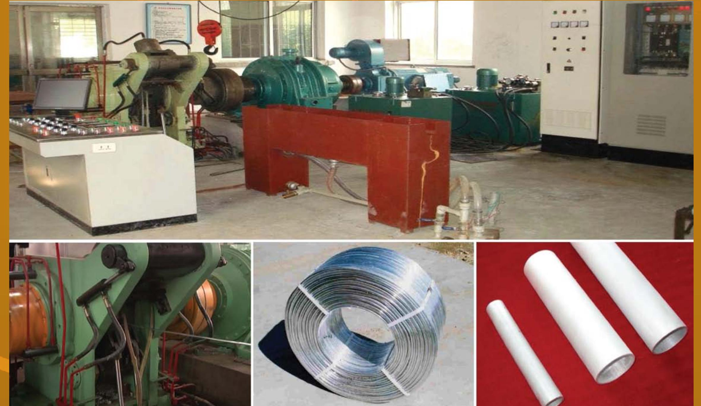
Continuous rheo-extrusion equipment and aluminum alloys wires and tubes prepared by continuous rheo-extrusion
