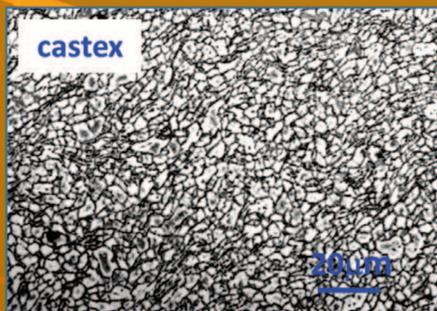
The continuous casting and extrusion technique (CASTEX) integrates the casting process with the extrusion process of severe shearing deformation. Mg- and Zn-based alloy bars and wires ( $\phi 2\sim 15$  mm) were successfully prepared by this process with high efficiency, low cost, and energy saving. The microstructures of Mg- and Zn-based alloys are effectively refined and their mechanical properties are remarkably improved.
